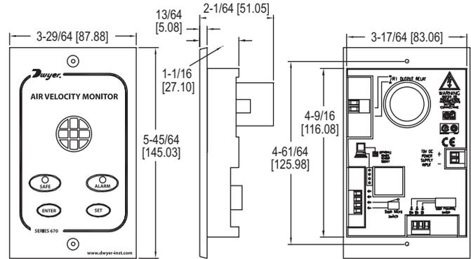
The **Model 670 Fume Hood Monitor** continuously senses air flow through the face of the fume hood, ensuring safe levels of fresh air are exhausting. The 670 provides a highly accurate hot wire sensor to detect very low flows common on fume hoods. The Model 670 comes with everything required to quickly install the unit including a mounting bracket, 24" of tubing for connecting to the inside of the hood wall and a 120 Volt AC power adapter.
