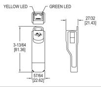
The Model MN-1 Mini-Node Communication Signal Converter is a low cost device that converts half duplex RS-485 serial communications signals into a signal that can be read by any computer with a USB port. The integral USB connector and RJ-45 connector reduces set up time by eliminating extra wiring. The Model MN-1 is powered via the USB connection which eliminates the need for an external power source. The compact size is great for field installation, control panels, and lab testing.
