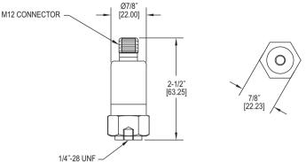
The **Model VBT-1 Vibration Transmitter** continuously detects the vibration in a system and monitors for unusual operating conditions and potential failure. The vibration is converted into an analog signal at the current output. The 2-wire loop power operation, combined with standard M12 micro cable connector and interchangeable mounting studs, make for a fast and reliable installation.
