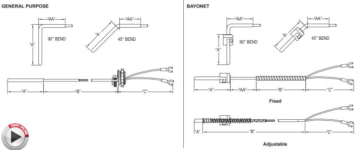
Series 4 & 5 General Purpose and Bayonet Type Thermocouples & RTD's tip temperatures can be as high as 842°F (450°C) for fiberglass insulated wire, and 392°F (200°C) for FEP insulated wire. Models can be specified with lead wires or head assembly construction. For higher temperatures see the Series R & 8 Mineral Insulated Probes.
