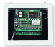
Master board stacked with channel expander
