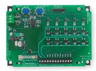
The Series DCT500ADC Low Cost Timer Controller is designed to provide continuous or on-demand cleaning for 10-35 volt powered receivers and pulse jet systems. It is available in either 4, 6, or 10 channels, and each unit is the same size, minimizing enclosure space and reducing overall system installation cost. For added safety, the control circuitry including the control inputs are isolated from the line voltage.
